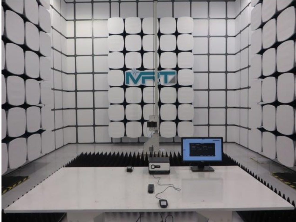
Description: Radiated Emission Test Setup for 18GHz ~ 25GHz
