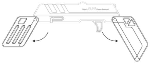
**4. Lock the handle: push the left handle to the right and push the right handle to the left in line with the arrow direction shown in the following picture**
