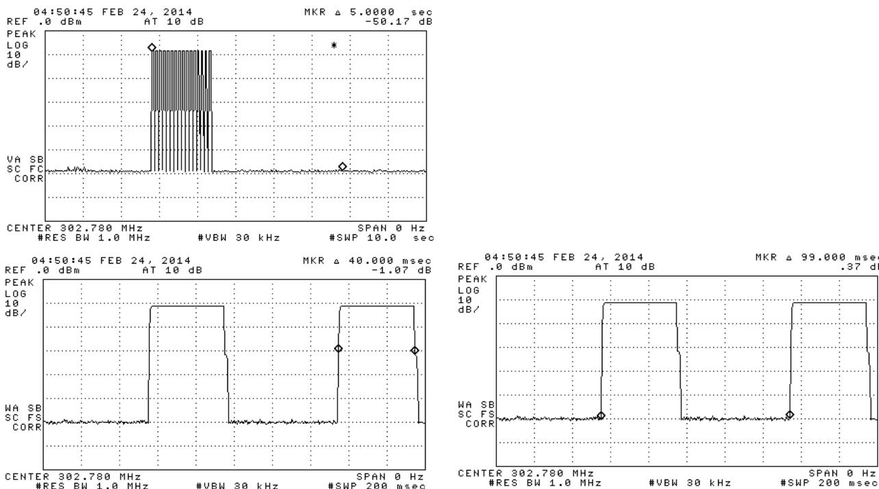
Figure 5: Pulsed Emission Characteristics (Duty Cycle).
