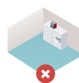
■ Devices deployment should avoid the metal, glass shield or other obstructions, and avoiding the corner.
