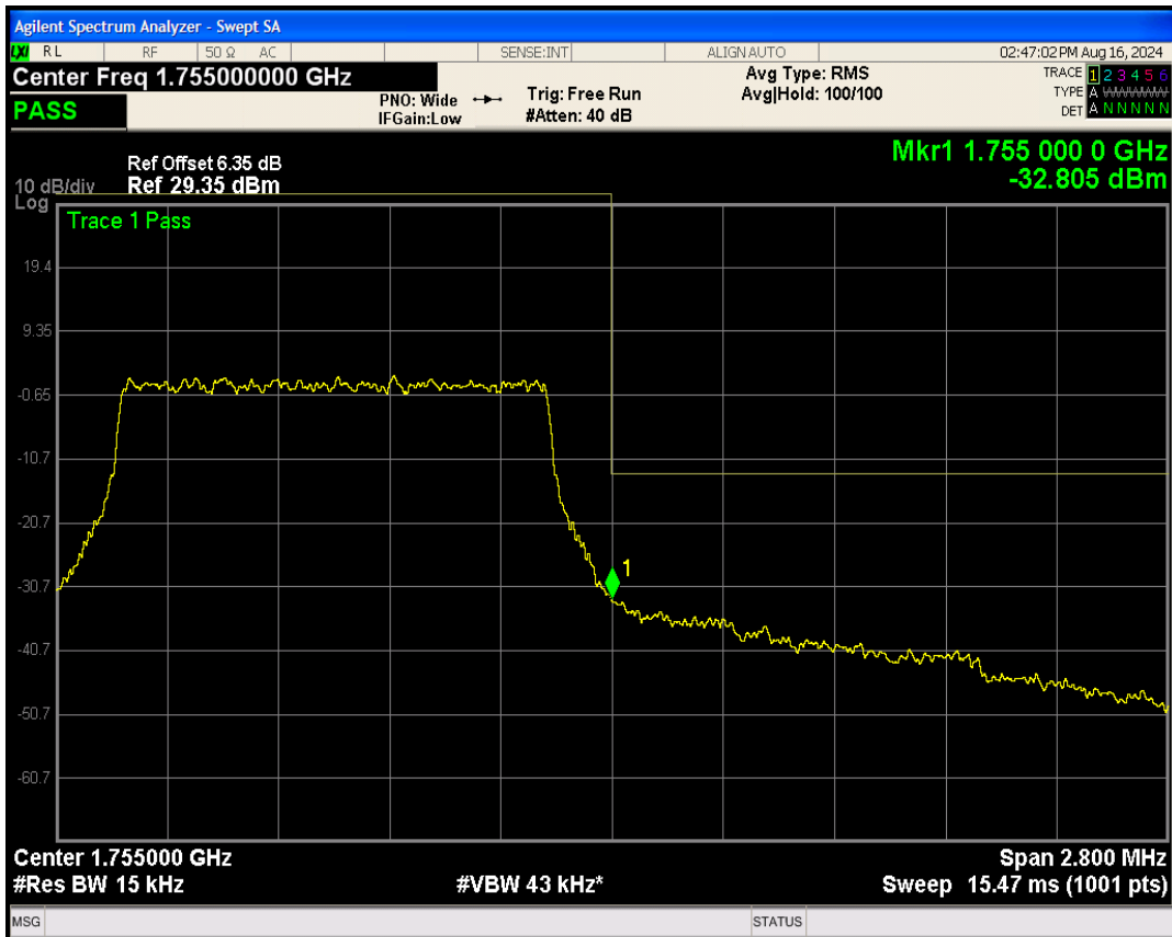
Band4 QPSK BW=3MHz Channel=19965 RB Size=15 Position=#0
