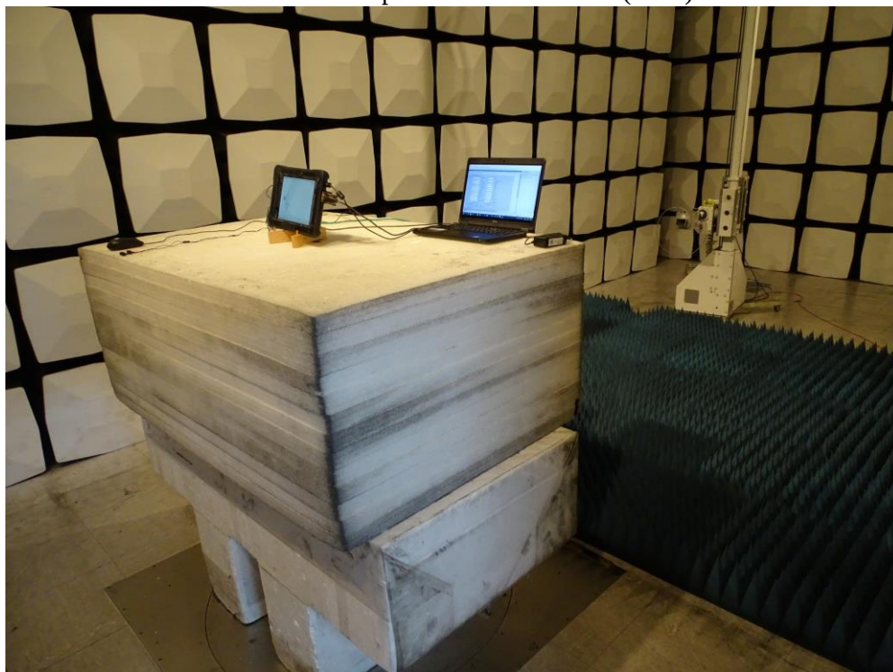
Back View of Spurious Emission Test (Horn)
