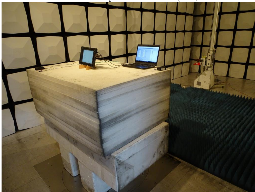
Front View of Spurious Emission Test (Horn)
