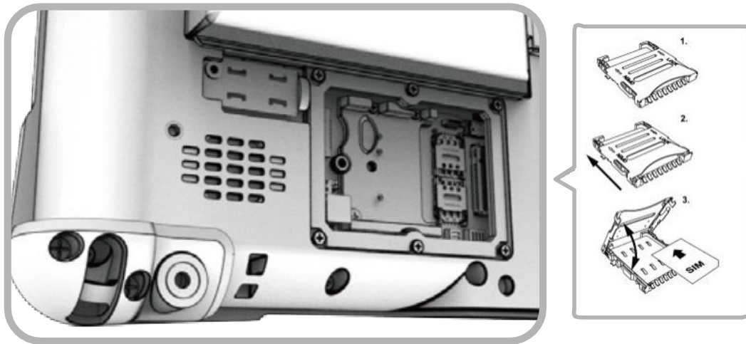
Figure 15. Installing the Nano SIM Card
