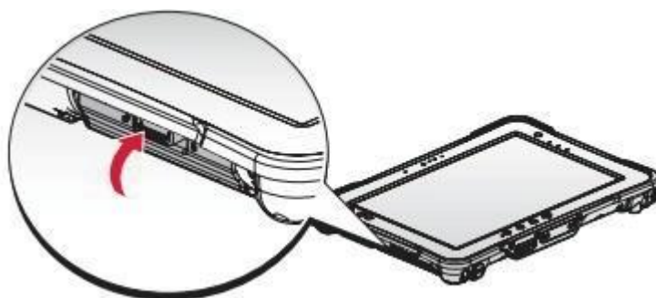
Figure 21. Installing the I/O Compartment Cover
