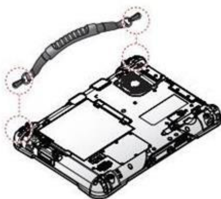
Figure 34. Connecting the Handle
