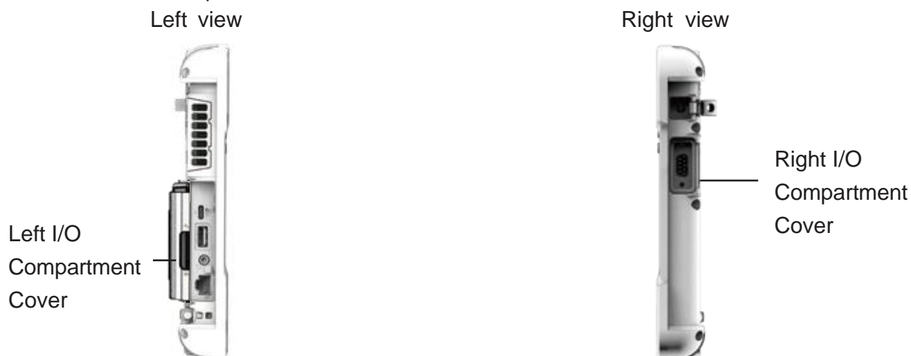
Figure 20. Side View: Locating the I/O Compartment Cover
