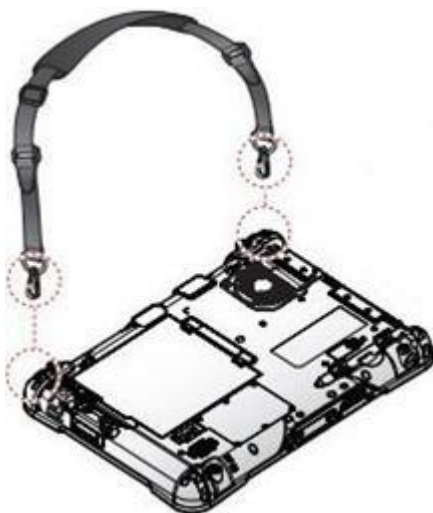
Figure 36. Connecting the Shoulder Strap
