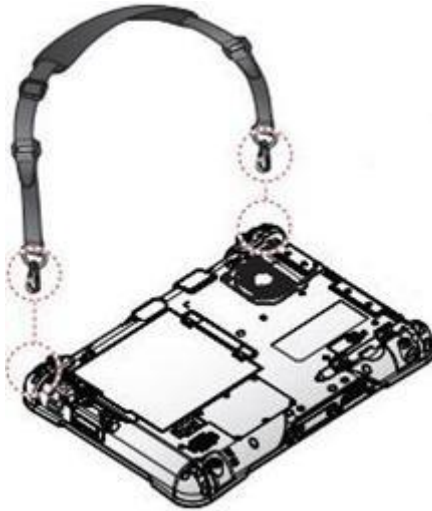
Figure 37. Removing the Shoulder Strap
