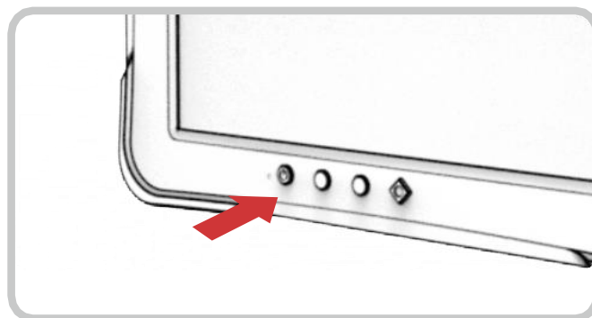
Figure 12. Power On the PX501
