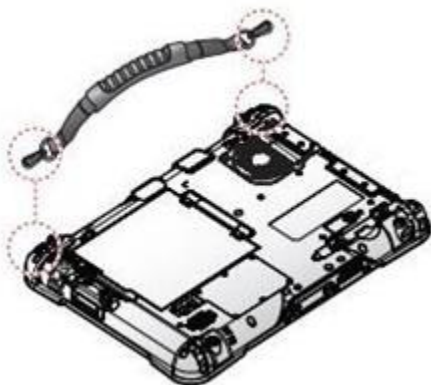
Figure 35. Removing the Handle
