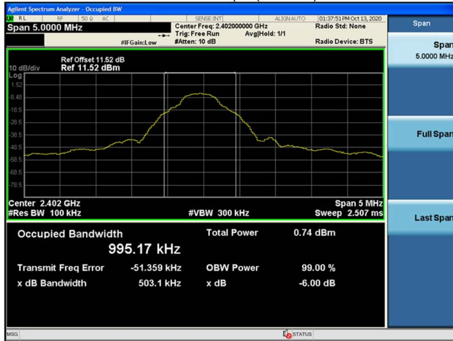
6 dB Bandwidth plot (Mid-CH 19)
