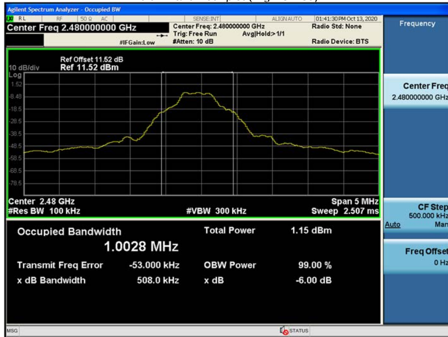
6 dB Bandwidth plot (High-CH 39)
