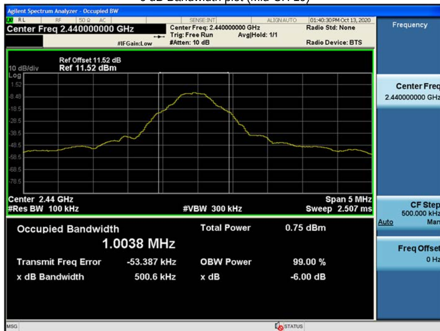
6 dB Bandwidth plot (Mid-CH 19)
