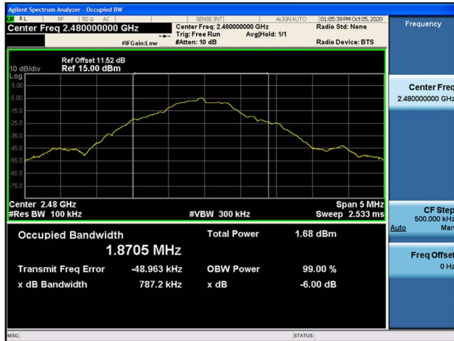
6 dB Bandwidth plot (High-CH 39)
