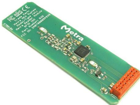
Metra Reader Module RFID ISO is designed to be build-in different Metra products. Reads ISO 15693, ISO 1443A and ISO 14443 B and compatible RFID media. It has two build-in blue LEDs for user signalization.
