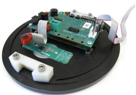
Example shows “Metra Reader Module RFID ISO” connected via 10 pole flat cable to host processor board. The cable length is limited to 20 cm. It was tested as such during compliance tests.
