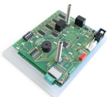
Example shows "Metra Reader Module RFID ISO" soldered directly onto the device's main PCB. Instead of using 10-pole flat cable the connector PINs are soldered directly (as if the cable length is equal 0). It was tested as such during compliance tests.
