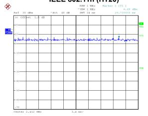
Duty cycle = 34.000 ms / 34.000 ms = 100% Duty Factor = 10 log(1/Duty cycle) = 0.00 IEEE 802.11n (HT40)
