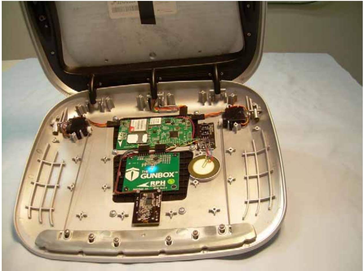
Location of the PCBs Except Power PCB
