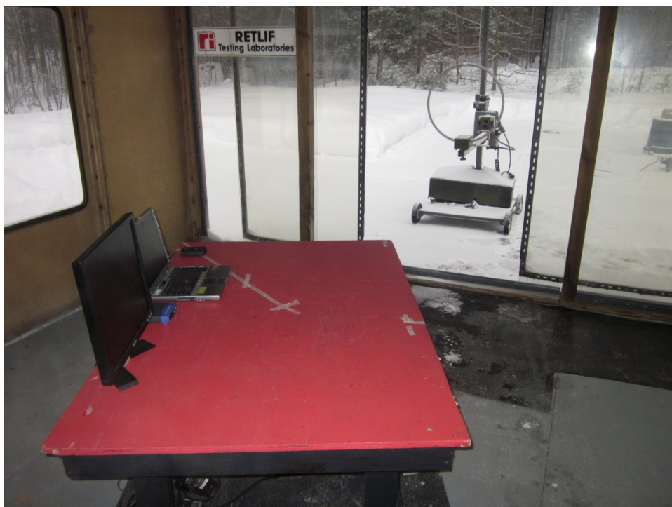
Test Setup, OATS, 9 kHz to 30 MHz
