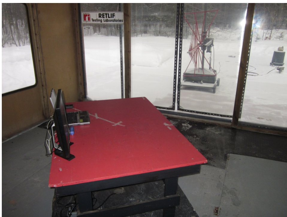
Test Setup, OATS, 30 MHz to 1 GHz, Vertical Antenna Polarization
