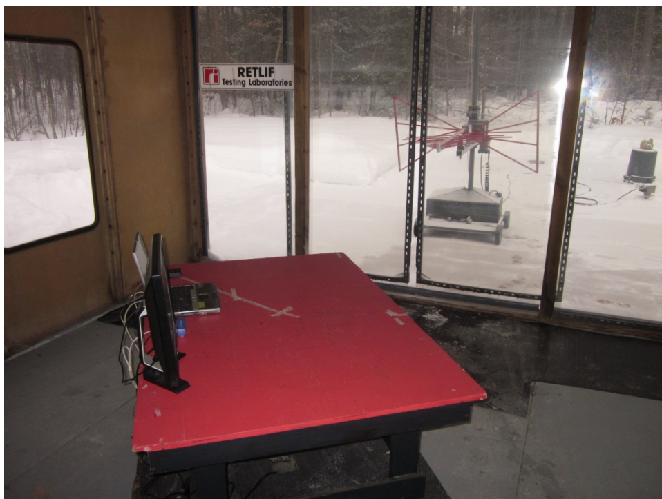
Test Setup, OATS, 30 MHz to 1 GHz, Horizontal Antenna Polarization
