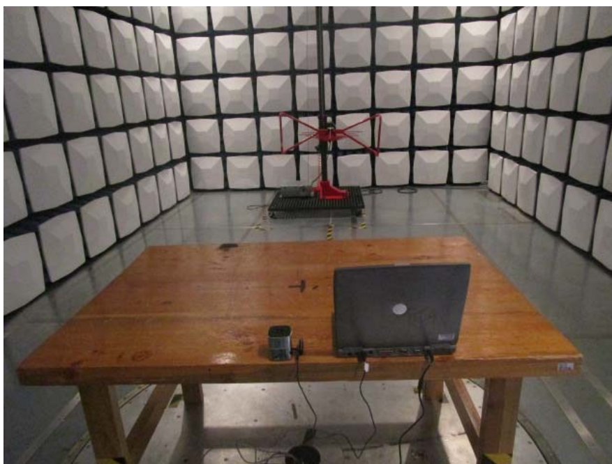
Radiated Emissions - Rear View (Below 1GHz)
