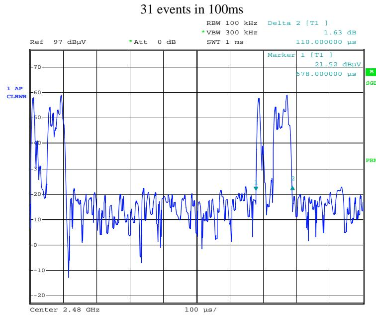
$$31 \times 0.678 \text{ } \mu\text{s} = 21.02 \text{ ms in 100 ms}$$
