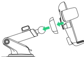
A. Connect the Mount Cradle with the Ball Joint.
