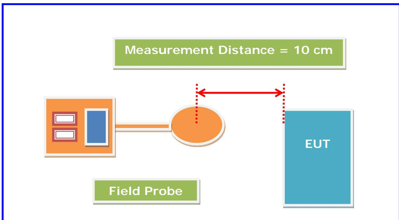
Measurements should be made from all sides and the top of the primary/client pair, with the 10 cm measured from the center of the probe(s) to the edge of the device.
