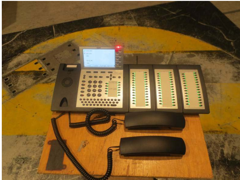
Figure 5: test setup for Radiated disturbances 1 GHz to 2 GHz – Operation mode 2 with AC/DC Adapter
