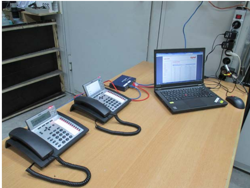
Figure 1: Test Setup Conducted Emissions (150 kHz – 30 MHz) – Operation mode 2 with AC/DC Adapter
