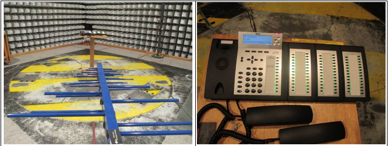
Figure 7-7: Test Setup Radiated Emission (30 MHz – 1 GHz) – Operation mode 1 with POE
