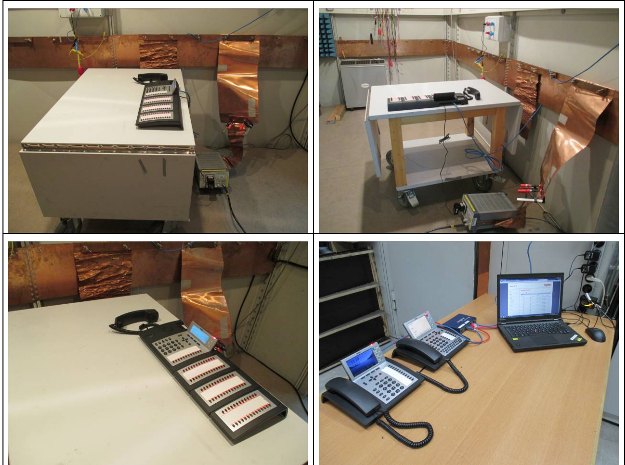
Figure 7-6: Test Setup Conducted Emissions (150 kHz – 30 MHz)
