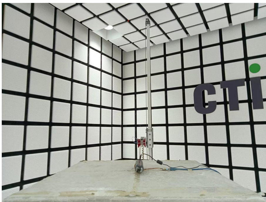
Radiated spurious emission Test Setup-2(Above 1GHz)
