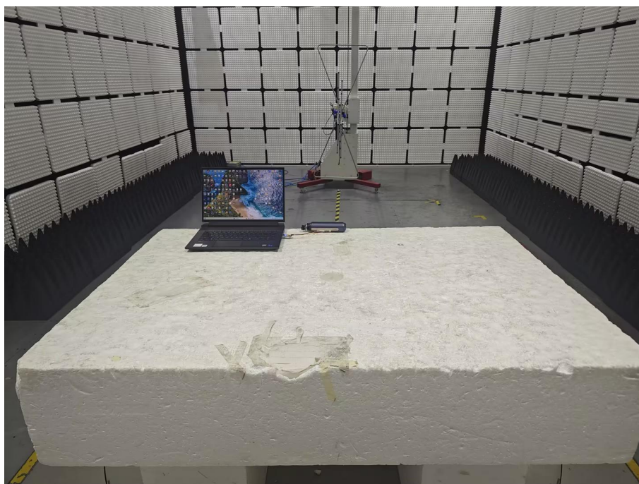
Radiated spurious emission Test Setup-1(Below 1GHz)
