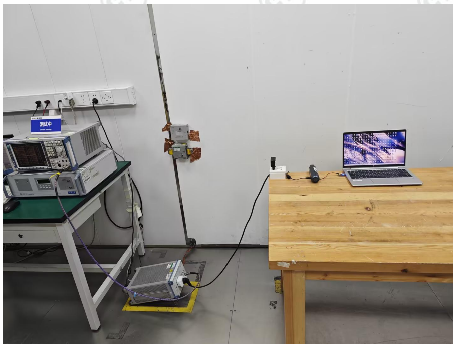
Conducted Emissions Test Setup
