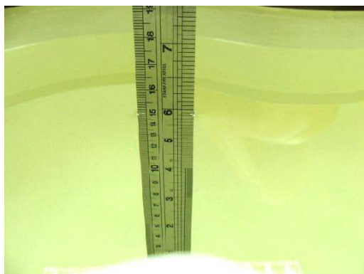
Fig 6.1 Photo of Liquid Height for Head SAR
