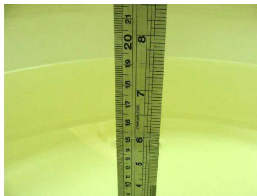
Fig 6.2 Photo of Liquid Height for Body SAR
