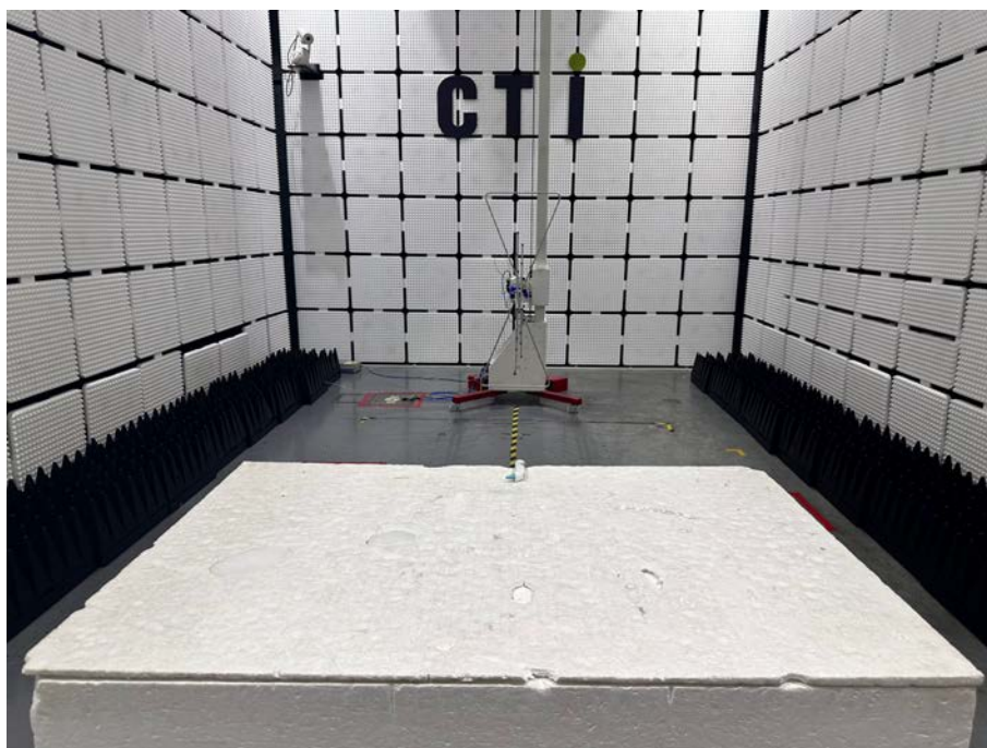
Radiated spurious emission Test Setup-1(Below 1GHz)
