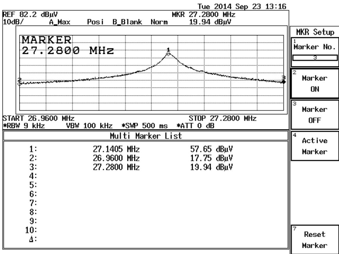
From above plot, at the bandedge 26.96 and 27.28MHz, are more than 38dB down from the 27.145MHz carrier. That mean the Operation frequency is within the band: 26.96 – 27.28 MHz and meets the requirement of Section 15.227(b)..
