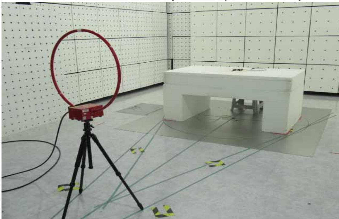
**Radiated Emission Set up Photos (Below 1GHz)**
