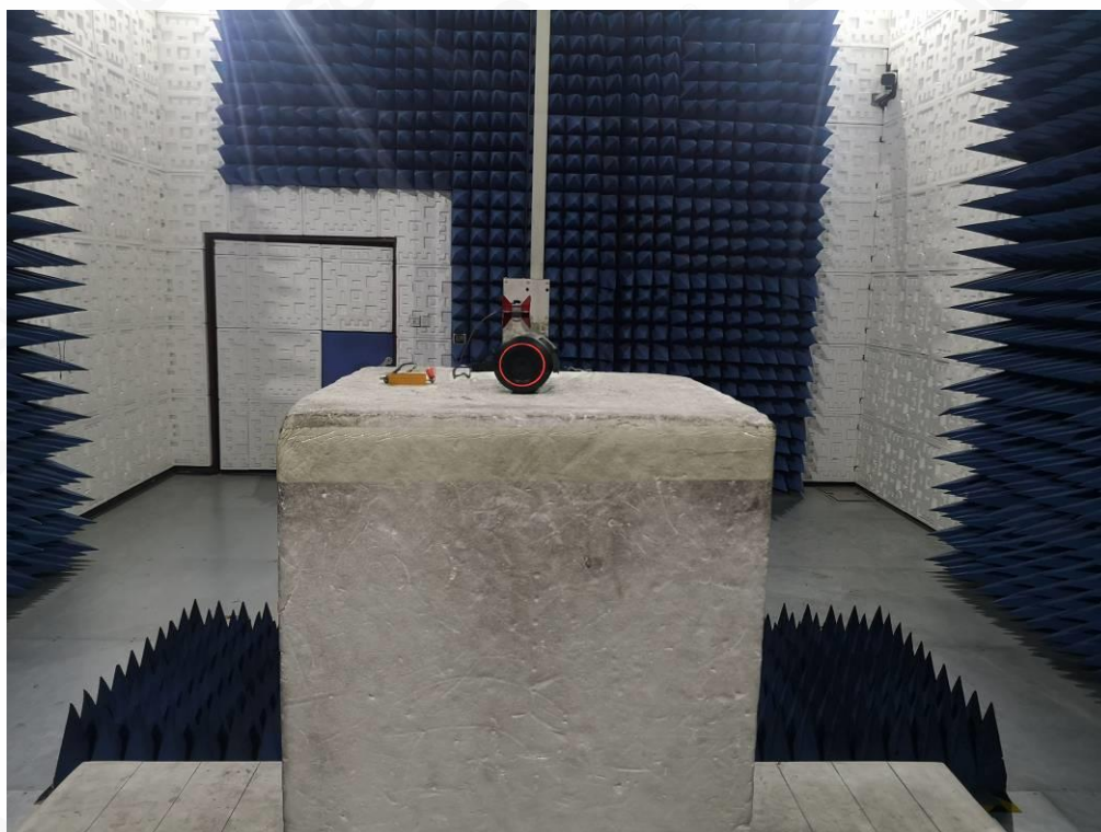
RADIATED EMISSION TEST SETUP ABOVE 1GHZ
