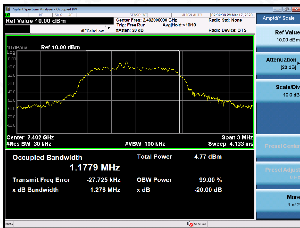
TEST PLOT OF BANDWIDTH FOR LOW CHANNEL
