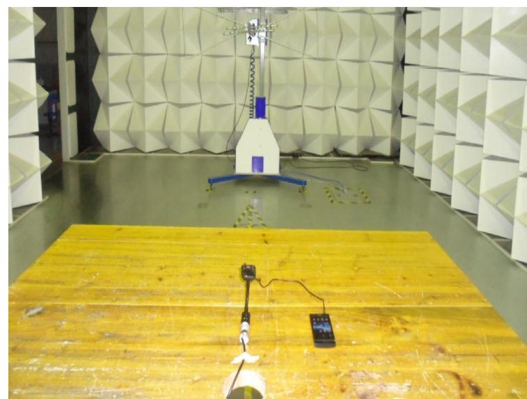
Test Mode: FM Transmitter Mode From 30-1000MHz
