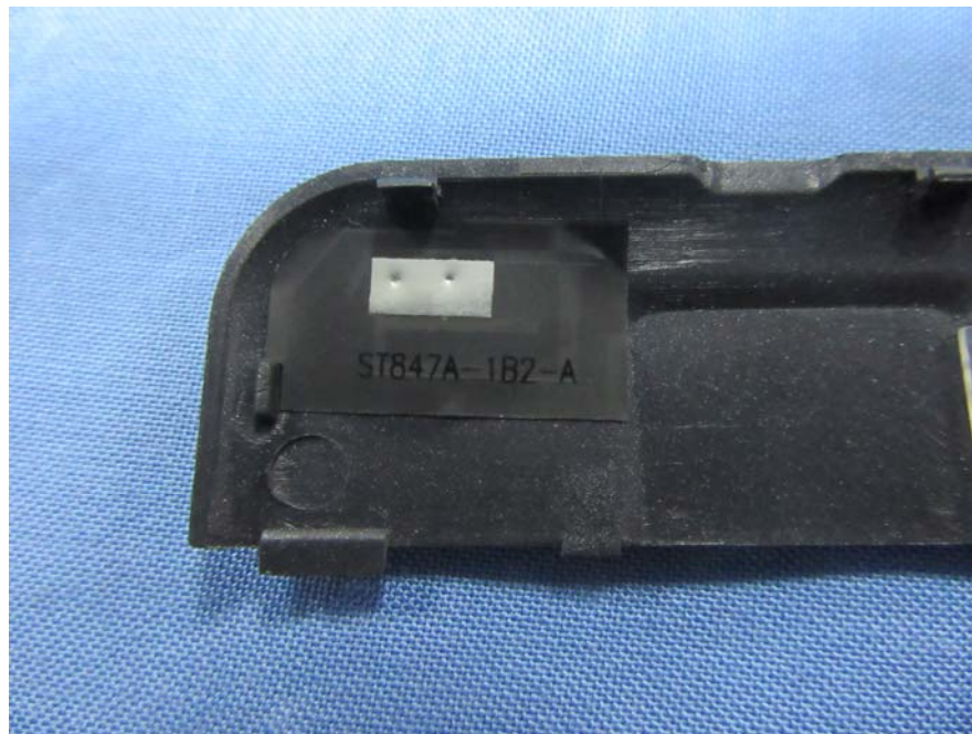
EUT – BT&WIFI Antenna View
