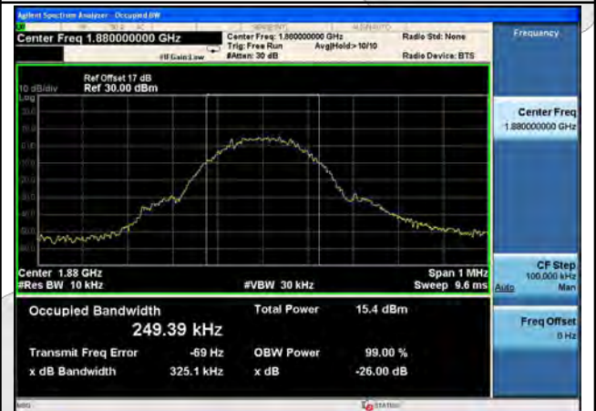
GPRS 1900 BW - Mid CH 1880MHz
