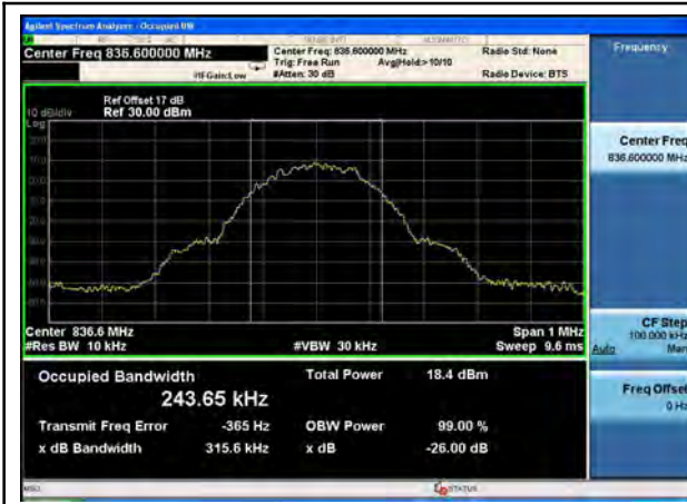
GPRS 850 BW - Mid CH 836.6MHz
