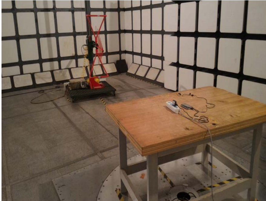
Radiated Emissions View (Below 1 GHz)
