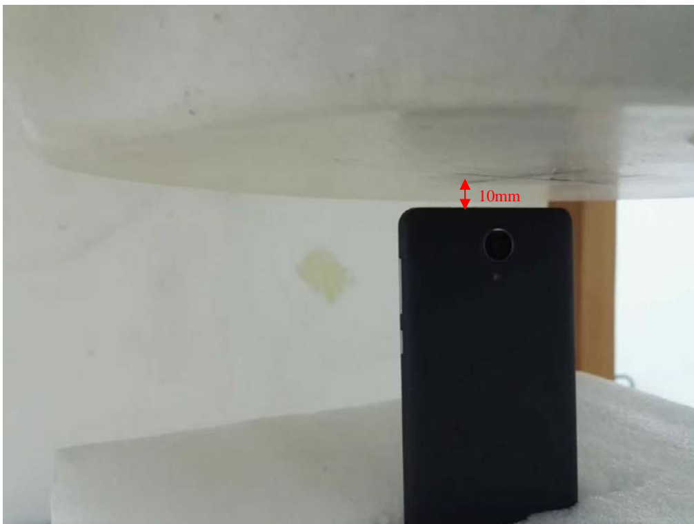
Body-worn Top Setup Photo (10 mm)
