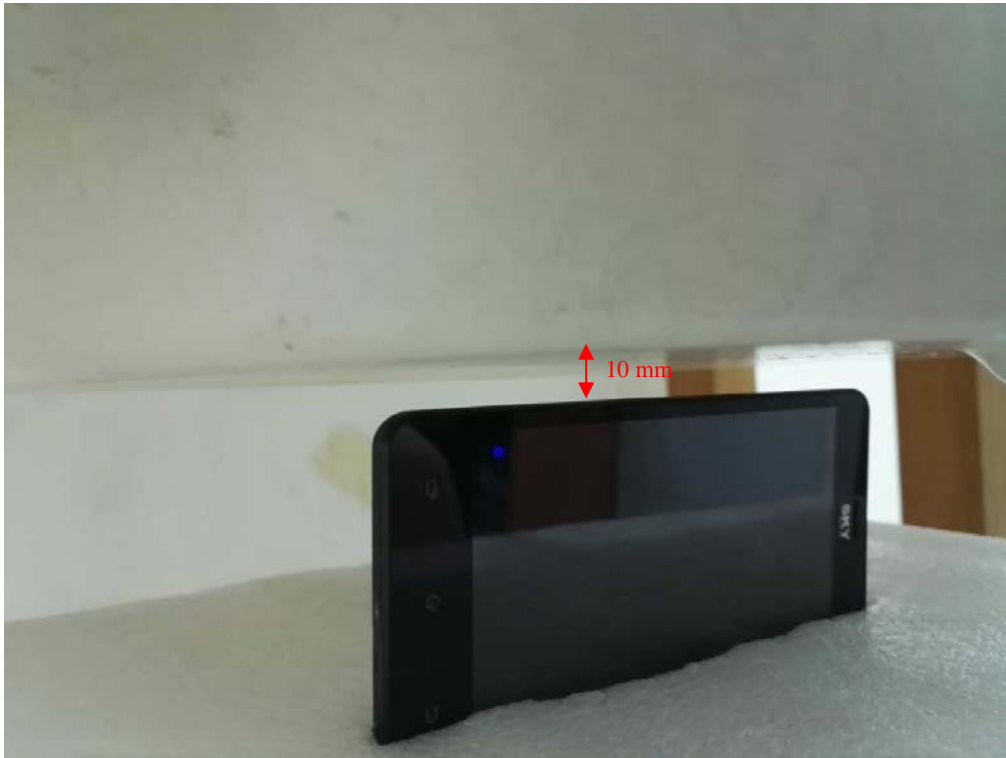
Body-worn Left Setup Photo (10mm)
