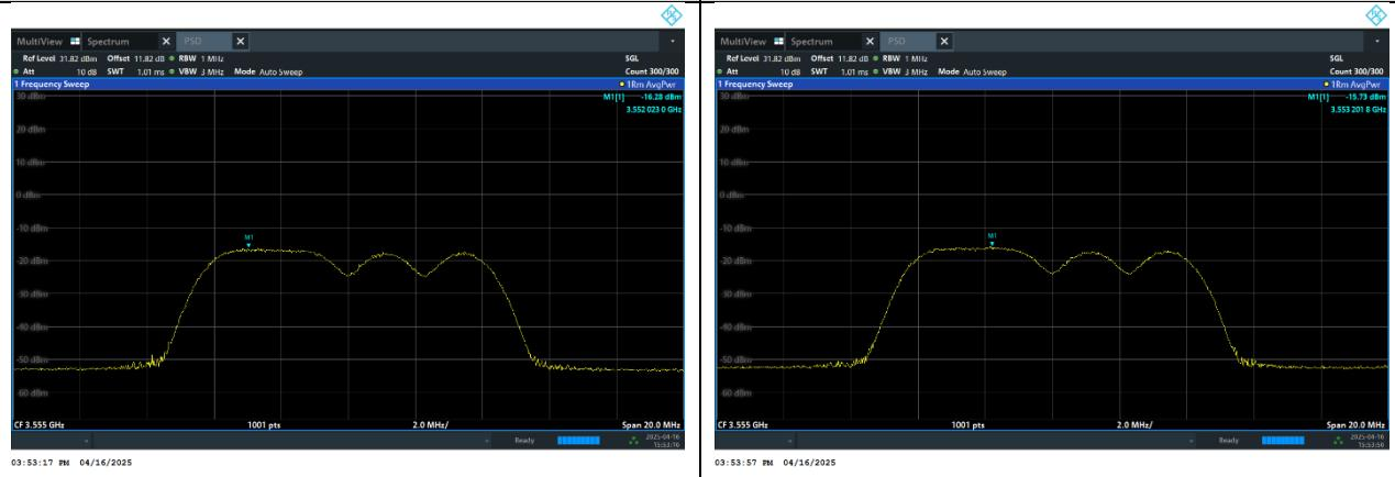
**SAS Granted MaxEIRP 23 [dBm/MHz]****UUT Center Frequency 3555 MHz, Bandwidth 10 MHz, Total EIRP PSD 21.72 [dBm/MHz]****Conducted PSD [dBm/MHz]****Polarization H****Polarization V**
