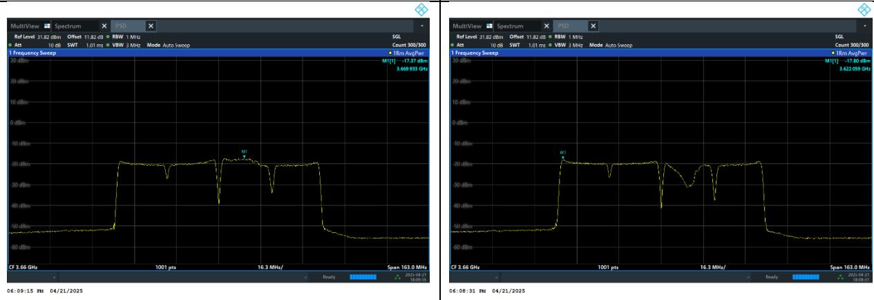
**SAS Granted MaxEIRP 37 [dBm/MHz]****UUT Center Frequency 3555 MHz, Bandwidth 10 MHz, Total EIRP PSD 36.07 [dBm/MHz]****Conducted PSD [dBm/MHz]****Polarization H****Polarization V**
