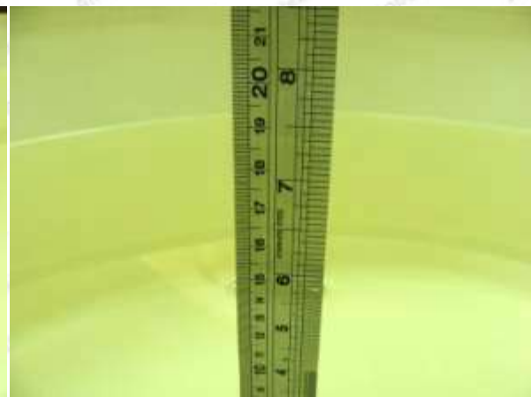
Photo of Liquid Height for Body SAR
