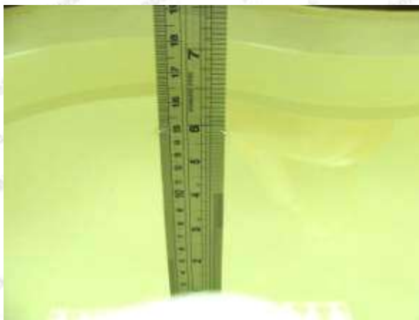
Photo of Liquid Height for Head SAR
