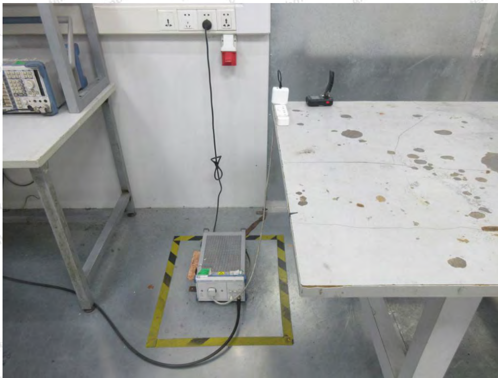
Photo of Power Line Conducted Emission Test
