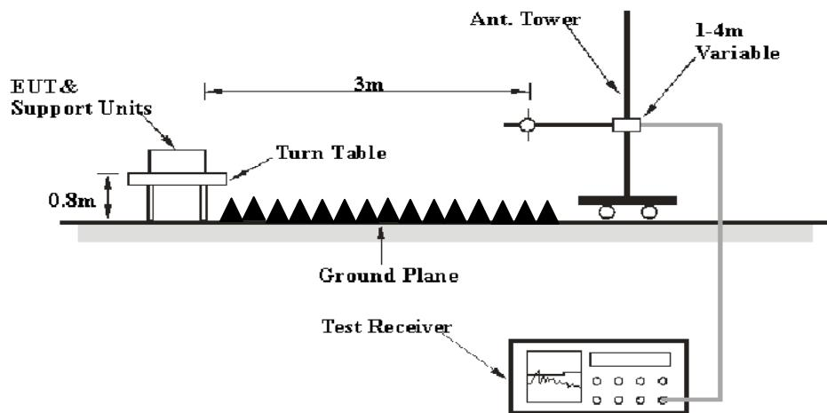
The radiated emission tests were performed at the 3 meters distance in chamber, using the setup accordance with the ANSI C63.4-2014. The specification used was the FCC Part 15.109 Class B limits.
