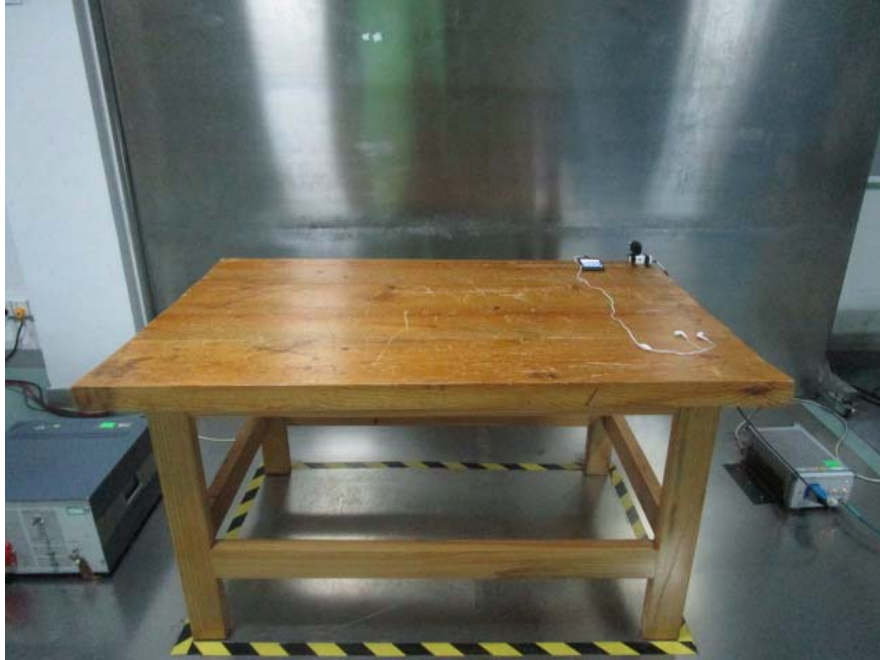
Conducted Emissions - Front View
