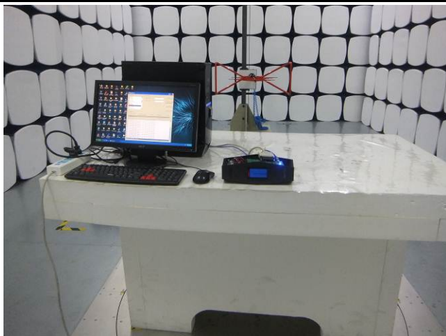
Radiated Spurious Emissions Test Setup Below 1GHz
