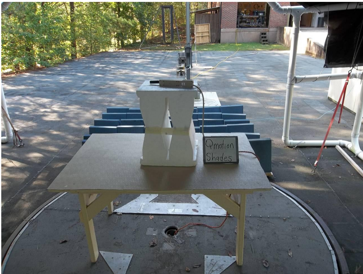
Figure 6. Radiated Emission Test Setup, above 1 GHz, Back
