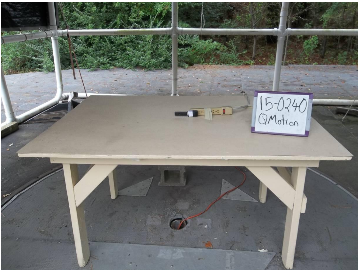
Figure 1. Radiated Emissions Test Setup, Front below 1 GHz
