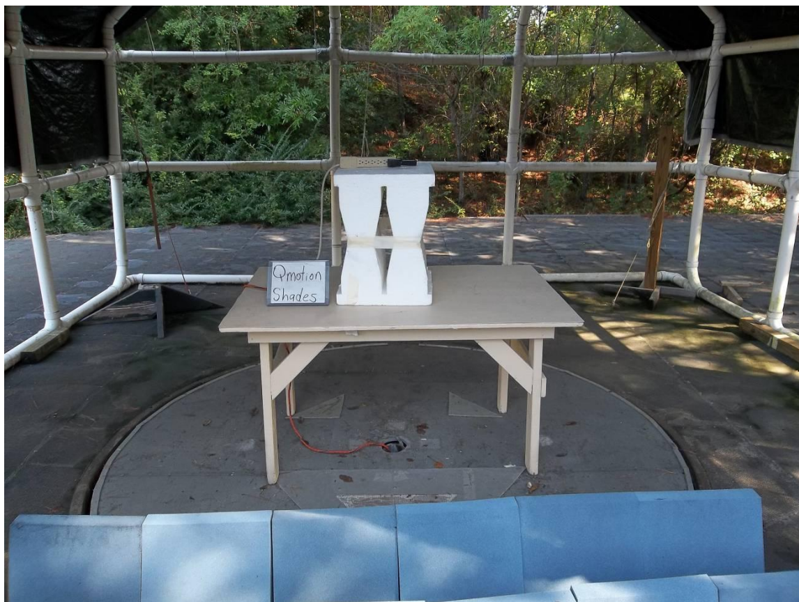
Figure 2. Radiated Emissions Test Setup, Front above 1 GHz
