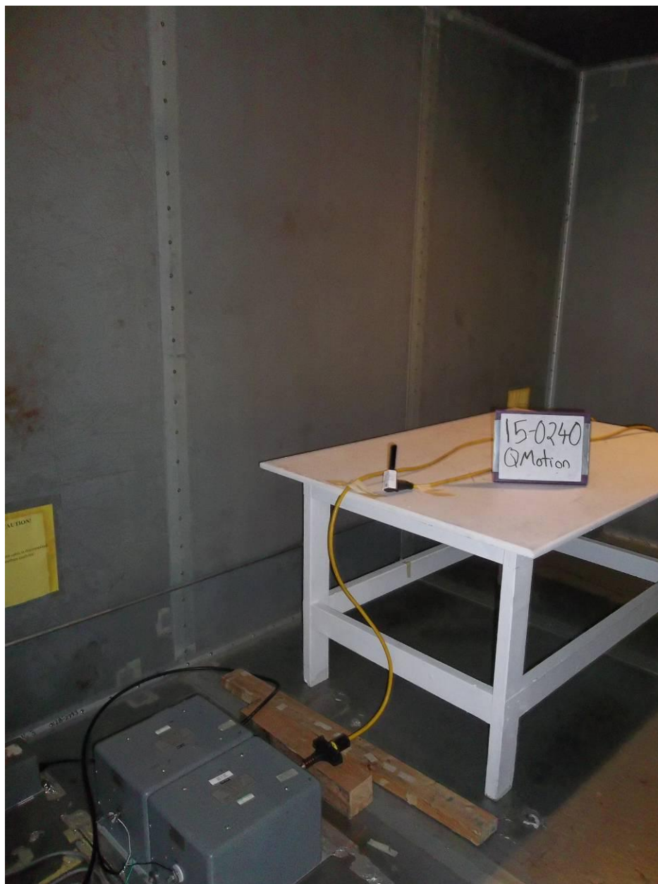
Figure 7. Conducted Emissions Test Setup
