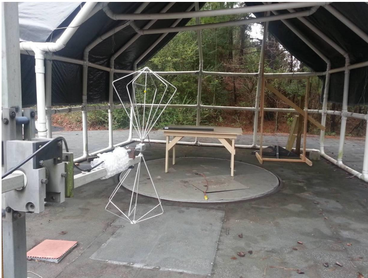
Figure 1. Radiated Emissions Test Setup, Front (Below 1 GHz)
