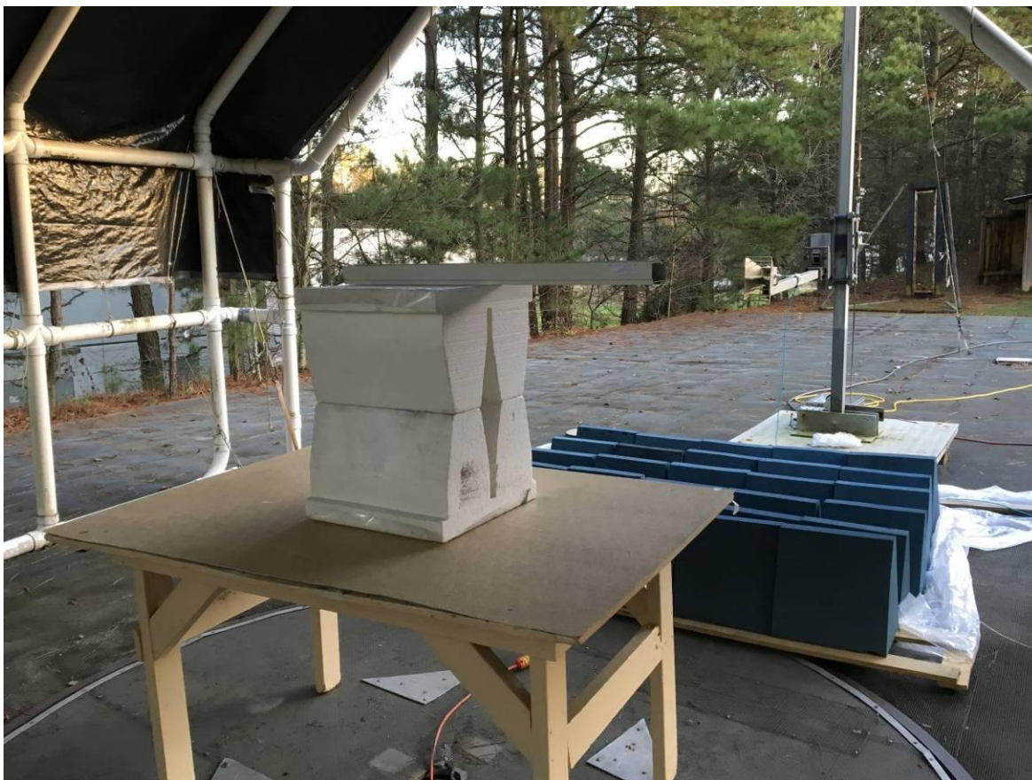
Figure 5. Radiated Emissions Test Setup, above 1 GHz, Back
