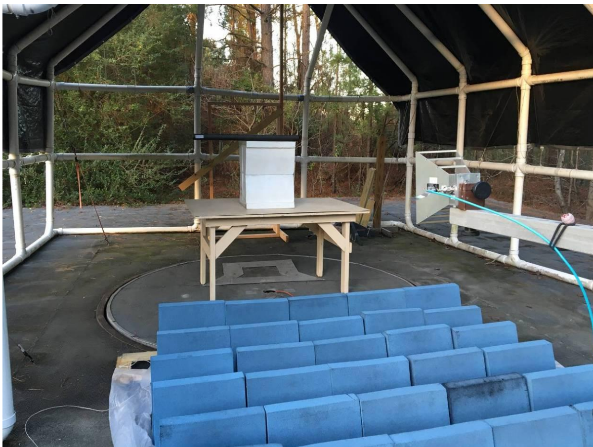
Figure 2. Radiated Emissions Test Setup, Front (Above 1 GHz)
