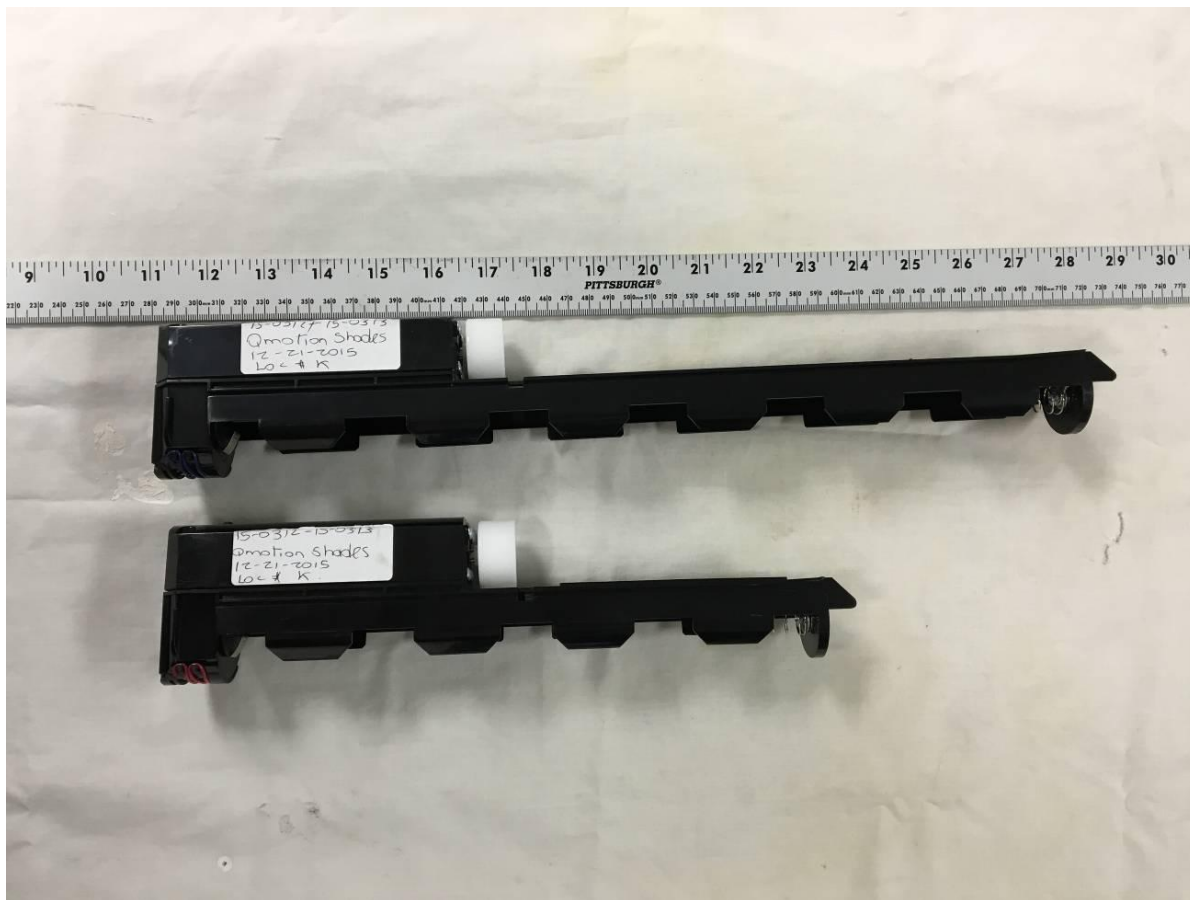
Figure 2. EUT/Motor Removed from Fixture (4-Battery and 6-Battery Models Displayed)
