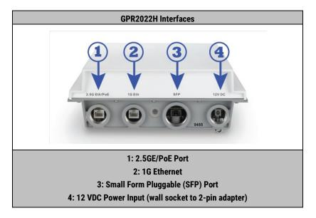
Interfaces are recessed at the bottom of the unit.
