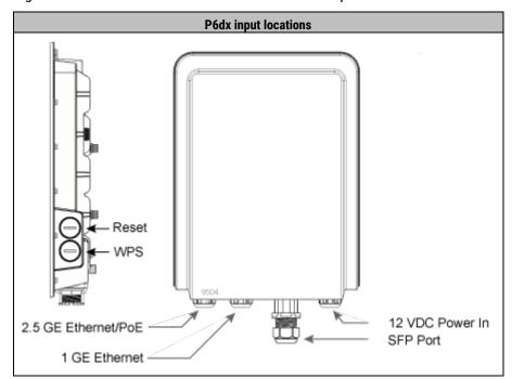
The fittings shown above are attached to the bottom of the p6dx enclosure in the order shown.
