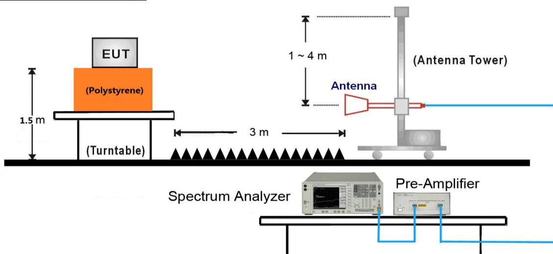
18GHz ~40GHz Test Setup:
