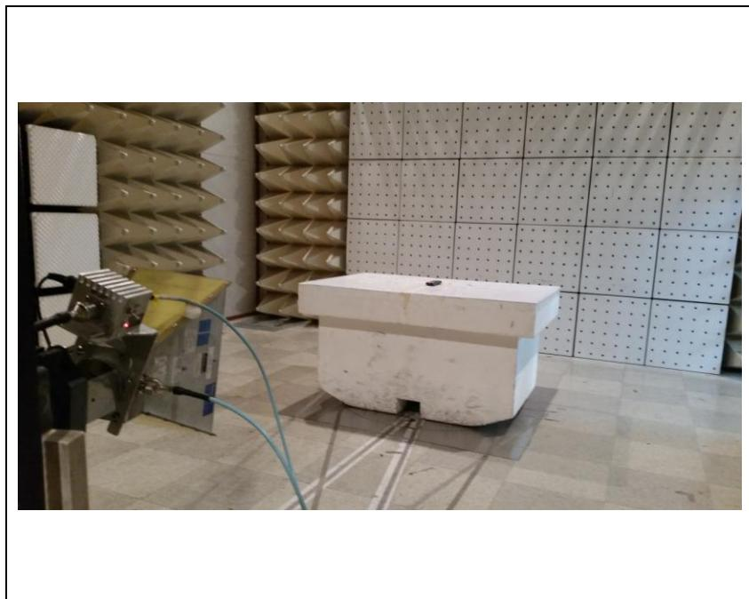
**C. Photo of Test setup (1 GHz ~ 4.5 GHz) : X-axis**
