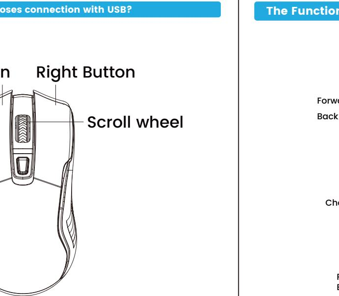
Press and hold the **left, middle, and right buttons** of the mouse for 3-5 seconds, then plug the USB into the computer.
