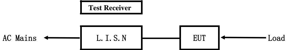
EUT: Equipment Under Test
