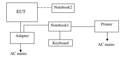
Notebook 2 connected to EUT by wireless connection, Notebook 1 connected to EUT though LAN port,
