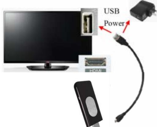
2. Switch on TV set and choose the corresponding HDMI signal source, MiraVision device name and MiraVision status will be played on TV screen as
