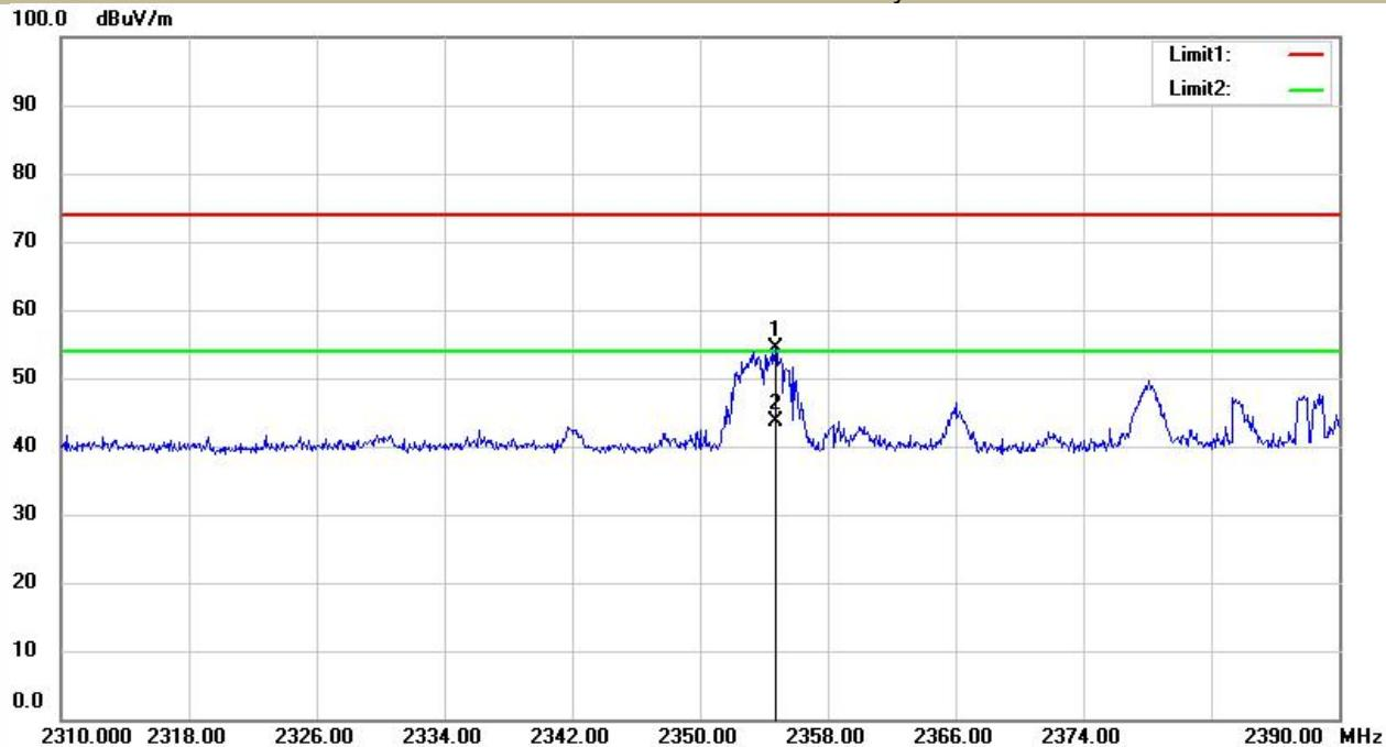
Test Mode Spurious Emission in Restricted Band 2310-2390MHz
