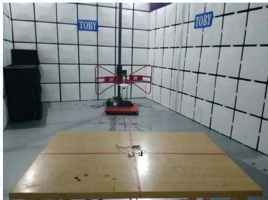
**Photo of Setup for Conducted Emission**
