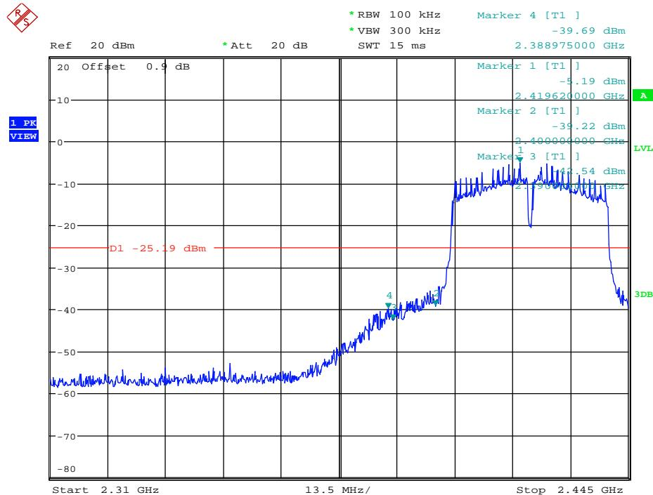
**Band-edge for RF Conducted Emissions\_11N40SISO\_2422\_Ant2**
