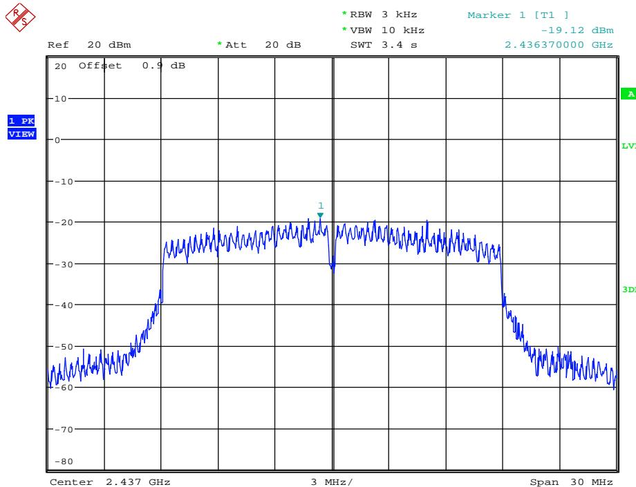
**Maximum Peak power spectral density\_11N20SISO\_2437\_Ant2**
