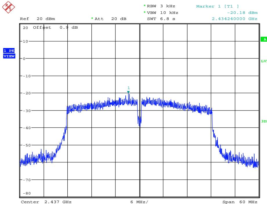
**Maximum Peak power spectral density\_11N40SISO\_2437\_Ant2**
