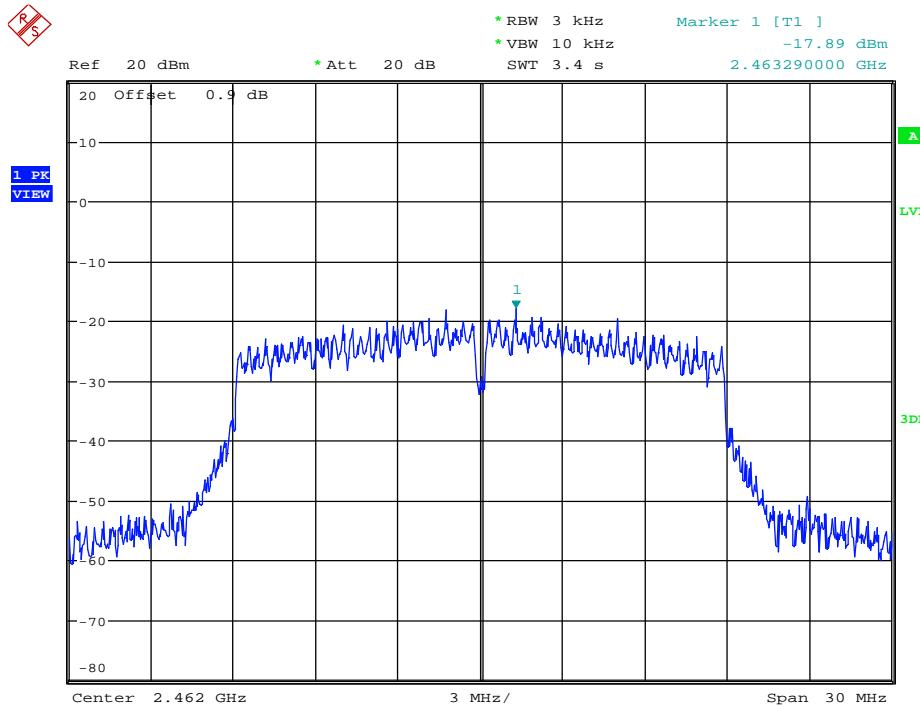
**Maximum Peak power spectral density\_11N20SISO\_2462\_Ant2**
