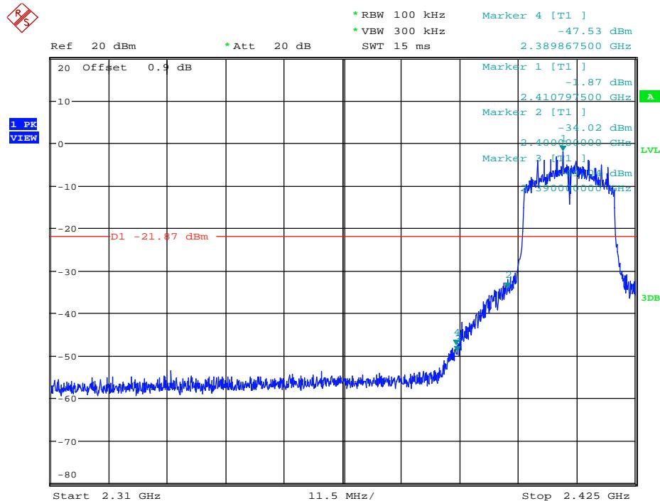
**Band-edge for RF Conducted Emissions\_11N20SISO\_2412\_Ant2**
