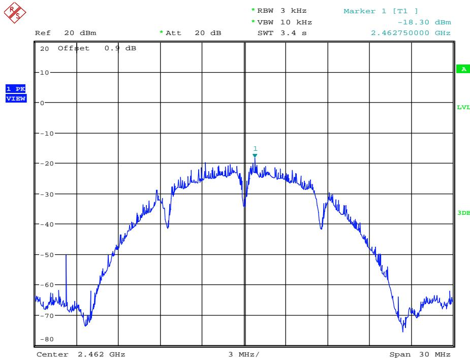
**Maximum Peak power spectral density\_11B\_2462\_Ant2**
