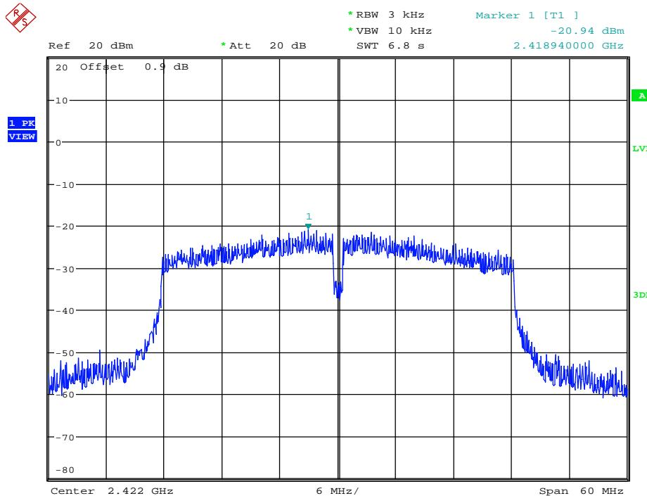
**Maximum Peak power spectral density\_11N40SISO\_2422\_Ant2**
