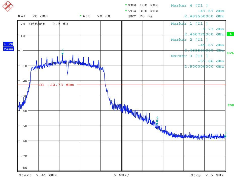
**Band-edge for RF Conducted Emissions\_11N20SISO\_2462\_Ant2**
