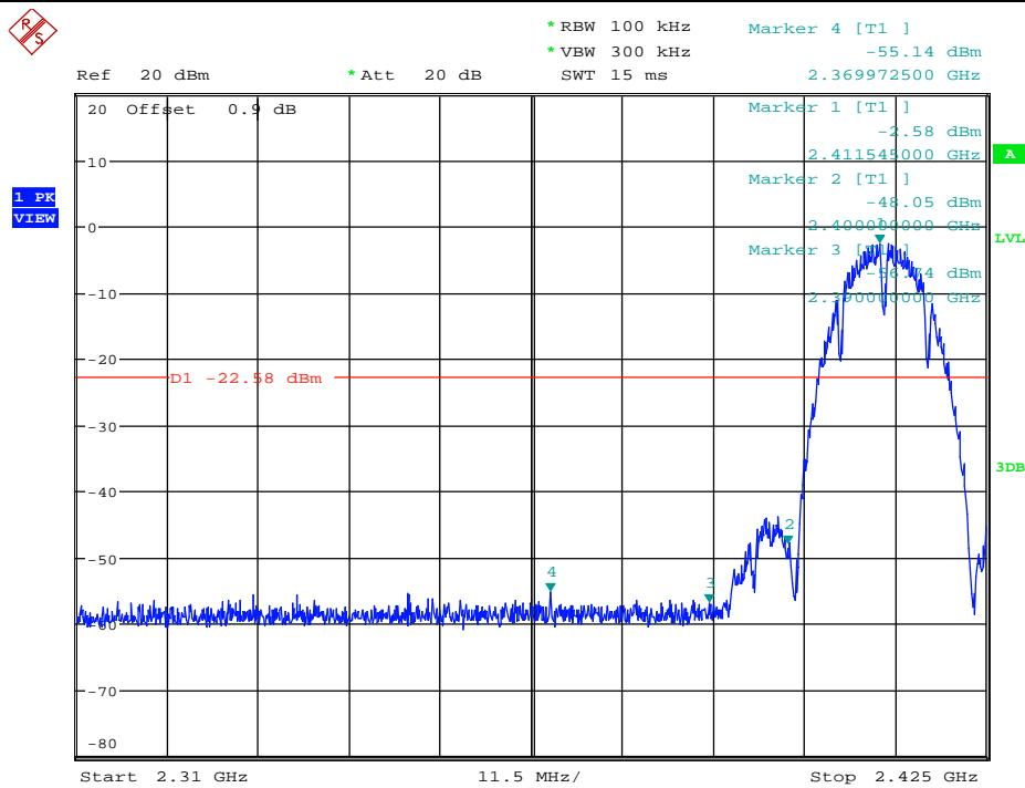
Band-edge for RF Conducted Emissions\_11B\_2412\_Ant2
