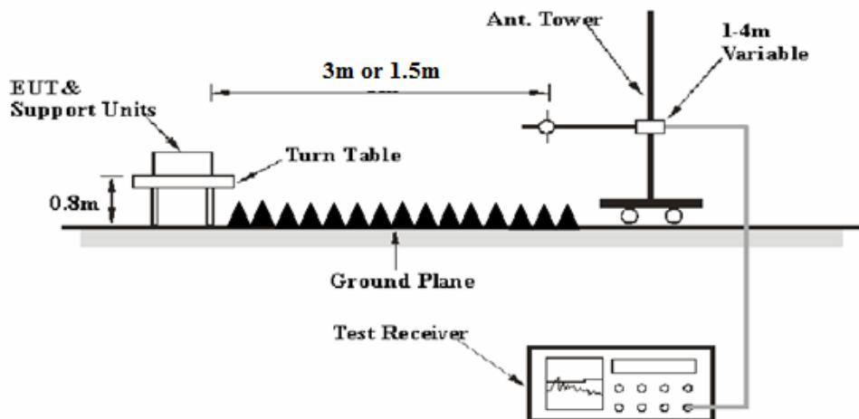
The radiated emission tests were performed in the 3 meters Semi-Anechoic Chamber, using the setup accordance with the ANSI C63.4-2003. The specification used was the FCC 15.209 and FCC 15.407 limits.
